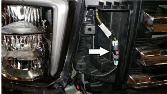
7. Mount the top bracket to the 18mm bolts. Hand tighten only. Keep the distance between the top bracket under 38" so the grill guard can be installed.
