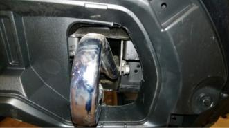
3. Remove the tow hook bolts and install the  $\frac{1}{2}$ " x 5" bolts. Mount the bottom bracket to the outside of the frame. Push the bracket upwards and tighten bolts and nuts.
