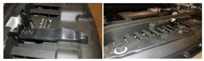
6. If vehicle is installed with a front camera, unhook the connector. The grille can then be removed by remove four 10mm bolts on top.
