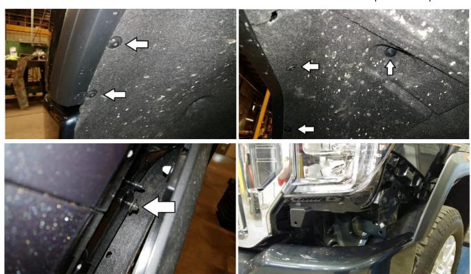
5. Remove the factory grille. Open the hood and remove the hood release latch by removing two T15 screws. Remove the nine plastic clips holding the plastic shield located above the grille.
