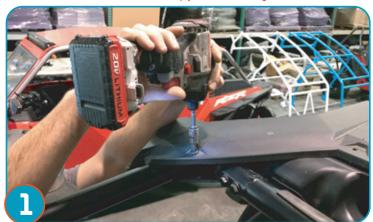
Remove four bolts from the plastics located on the top of the vehicle.
