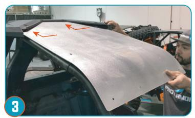
Place Pro Armor stock roof onto the vehicle and sliding the roof under the roof plastics, lining up bolt holes at the rear of the roof.
