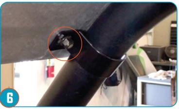
Using the provided (2) clamps and (2) hex bolt/nuts to secure the front of roof to stock cage as shown.
