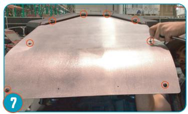
Tighten down all (8) bolts making sure roof is firmly secured to the vehicle.
