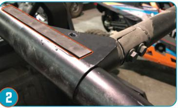
Apply the provided foam padding strips to the top of the stock cage.
