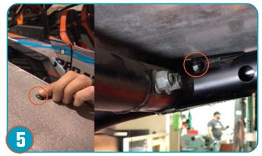
Using the provided hex bolts apply bolt and nut to middle location of roof on each side of vehicle/roof.
