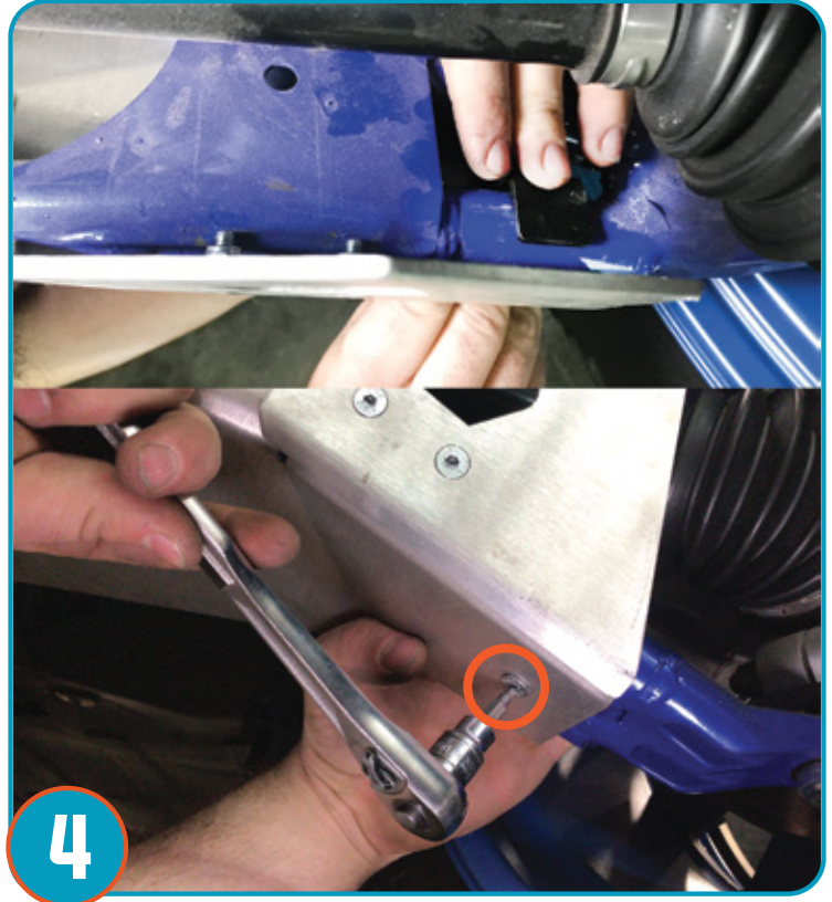
Position the small mounting bracket, over the front A-Arm and secure to A-arm Guard, using one (1) 16mm bolts, as shown. REPEAT STEPS FOR OPPOSITE A-ARM GUARD.
