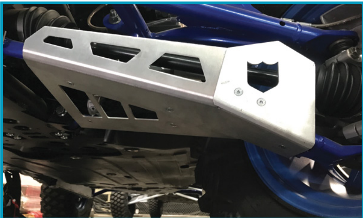
Position the small mounting bracket, over the front A-Arm and secure to A-arm Guard, using one (1) 16mm bolts, as shown. REPEAT STEPS FOR OPPOSITE A-ARM GUARD.
