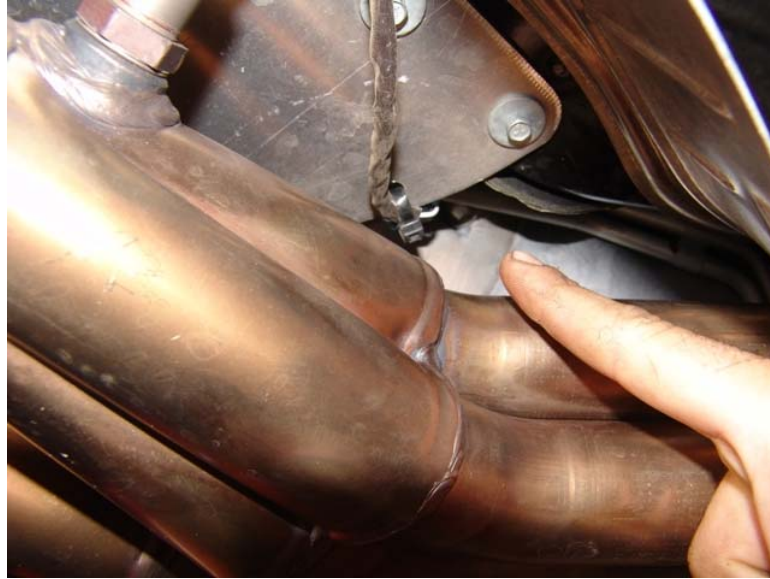
Figure 1: Front O2 sensor wire hold down.
