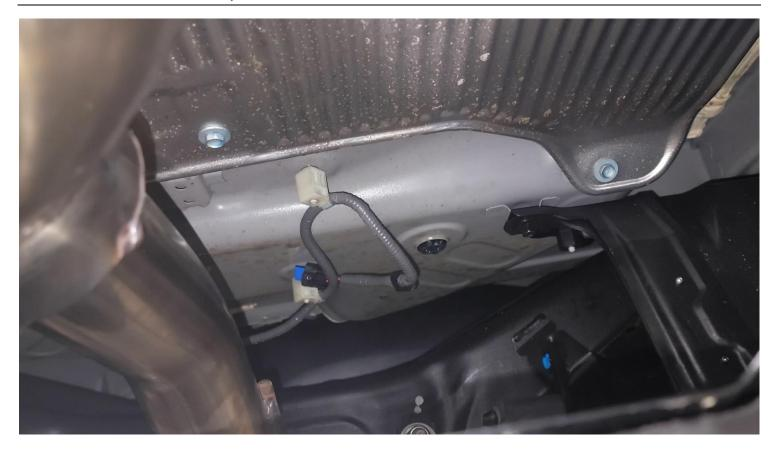
**Step #4** – Secure the electronic valve connector in a safe spot away from any moving components.
