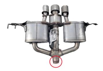
**STEP #1:** Locate the cut point on the under-axle tube. Mark the cut point 5/8" of an inch before the weld on the stock exhaust. (Circled in red above, and shown below)
