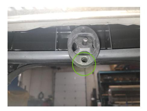
**Step #5** – Tighten the exhaust clamp connection between the factory exhaust and your new Street Race Axle Back.
