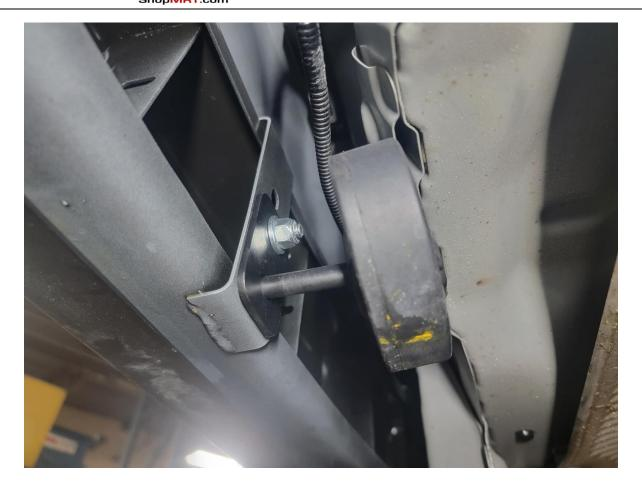
Step #3 – Slide the exhaust hanger located over the tips into the newly installed rubber isolator. (Circled in green below)
