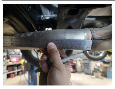
**Step #2:** Use a Sawzall to cut the factory exhaust.
