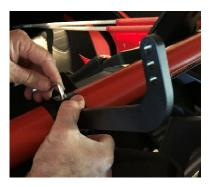
**STEP 3.** After Roll Bar Clamps (1) are installed, measure gap between the Metal Brackets (5) and set at 9.5 inches and tighten bolt. Insert the Duct Adapter (8) inside the vehicles air intake prefilter. Then install the vehicle air intake prefilter back into the vehicle. Place a Hose Clamp (2) over the Flexible Hose Duct (9) and insert onto the Duct Adapter (8) and tighten with Philips screwdriver.
