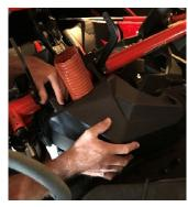
**STEP 5.** Install Particle Separator (1) onto the Metal Brackets (5) on the left and right-side using Screw (6) and Washer (4) and a 3/16" allan wrench to tighten. Washer **MUST** be between the Metal Bracket (5) and Particle Separator (1). If the washer is placed under the head of the Screw (6) the Particle Separator will rotate freely and may cause damage.
