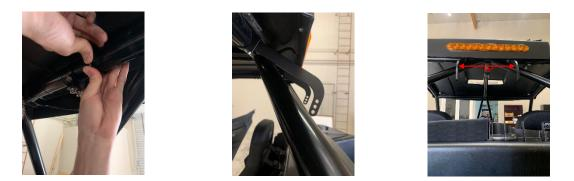
**STEP 6.** For upper roll bar installations use Step 5 with Metal Brackets (5) facing down. Install Particle Separator (1) onto the Metal Brackets (5) on the left and right-side using Screw (6) and Washer (4) and a 3/16" Hex Key to tighten. Washer **MUST** be between the Metal Bracket (5) and Particle Separator (1). If the washer is placed under the head of the Screw (6) the Particle Separator will rotate freely and may cause damage.
