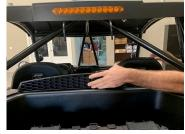
**STEP 3.** Measure across the long way of intake cover and mark at 15". From the 15" mark measure across the intake cover and mark with pen at 3 3/8". Were the two measurements intersect is the middle point for the intake hole. Cut a hole using a 3.75" diameter hole saw. Install included rubber stripping around the hole on the panel. Ensure to reinstall air intake cover onto vehicle before you proceed to STEP 4.
