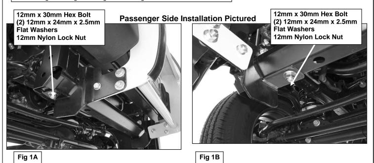
07-15 Passenger side Frame Mounting Bracket bolts to the outer mounting location (pictured with Grille Guard in position for example only)
