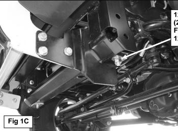
12mm x 30mm Hex Bolt (2) 12mm x 24mm x 2.5mm Flat Washers 12mm Nylon Lock Nut
