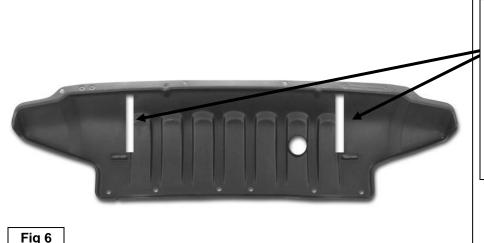
**Once the Mounting Brackets** have been installed and checked for alignment, hold the splash guard up into position and mark the cut area on the inside of the guard. Start with a small opening and slowly enlarge the opening to get the best fit around the brackets. Area cut from guard pictured for example only. (Interior view)
