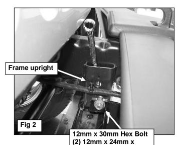
2.5mm Flat Washers 12mm Nylon Lock Nut (Install through opening in bottom of upright)
