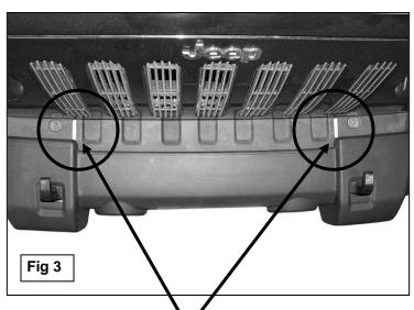
Reinstall the fill panel and mark the cut area on the inside of the fill panel straight up from the frame upright. Start with a small opening and slowly enlarge the opening to get the best fit around the brackets. Area cut from fill panel pictured for example only.
