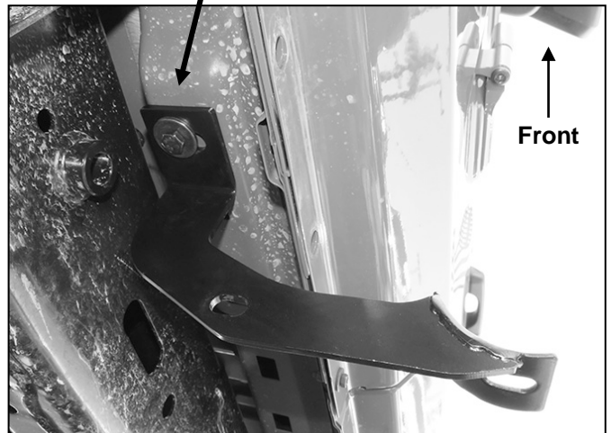
(Fig 4) Driver/left front Mounting Bracket installed
