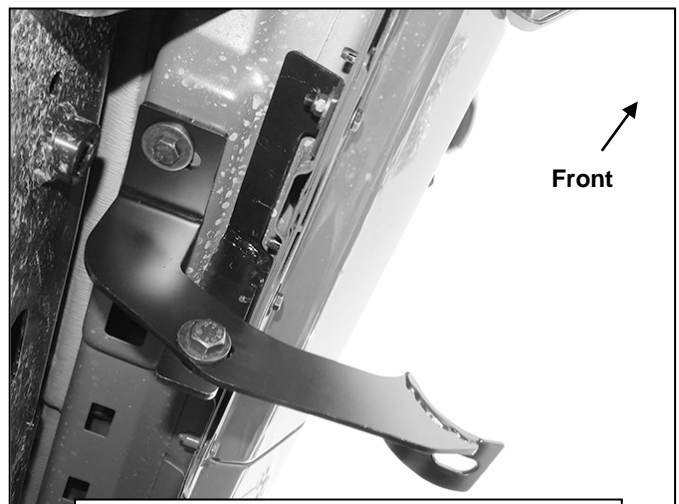
(Fig 6) Driver/left front Brackets installed
