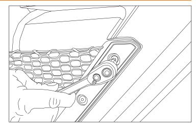
2. Position Door Panel Pocket to line up with the OE holes. Install using the OE hardware.
