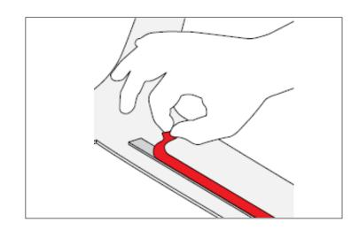
5. Firmly hold item in proper mounting position while pulling the exposed plastic liner to completely remove. Maintain pressure on installed item for 60 seconds to ensure proper contact. Full adhesion occurs within 24 hours of application.
