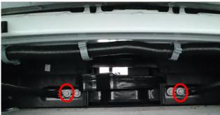
Fit the two U nuts to the front lower rails (inner holes) as per image.
