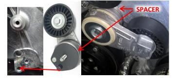
Fit the new idler pulley supplied to the boss above the
