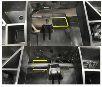
Remove the outer 2 screws from the tie bars.
