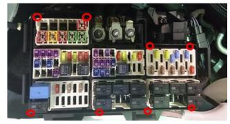
Now that the fuse assembly has been removed, remove the relays in the front right outer section. Now remove the white locking plate as shown in image.
