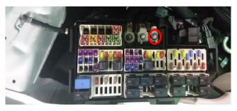
The earth wire is now secured under the screw located behind the ECU.
