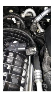
Connect the red, green, black, and yellow JB4 patch wire connectors to the stock manifold sensor and stock connector.
