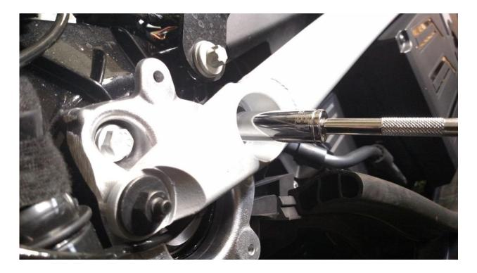
Remove the stock intake filter assembly which Is integrated into the engine cover.
