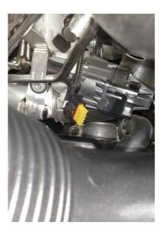
Plug the JB4 harness in to the wastegate controller and plug the stock connector in to the JB4 harness for both turbos. Note: There is no particular order.
