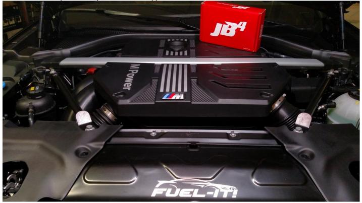
Open the hood and place your key far enough from the car not to wake it up, and wait 20 min for the vehicles computer to go to sleep. If you open a door the ECU will wake up. You can also disconnect the negative terminal on the battery.
