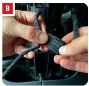
Route the Data Wiring Harness along factory wiring to the driver side kick panel area
