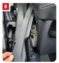
To remove the driver door sill panel you will need to remove the frunk release handle.
