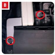
STEP 2: With the DSP/Amplifier Unit now mounted in place, locate and remove a 10mm bolt from the factory ground point above the driver side kick panel (A). Install the terminal end of the Ground Cable on to the factory ground point being sure to not leave off the factory ground wire (B). Using the supplied zip ties, secure any installed wires up and out of the way.
