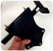
Install the two bracket assemblies onto the vehicle. Bracket "2/4/5" installs on the STEP 7: passenger side of the vehicle. Use the original 15mm bumper bolts that were previously removed to secure the assembly into place (A). Bracket assembly "1/3" installs on the driver side of the vehicle. Use the original 15mm bumper bolts that were previously removed to mount the bracket into place (B).
