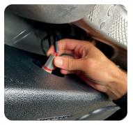
**STEP11:** Finally, remove two #2 phillips screws from the under body panel that was removed from the underside of the vehicle. Install the two Borla Speaker Grills (BOR-FME21G) and secure them to the panel using the previously removed phillips screws.
