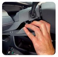
With the bottom steering wheel cover removed, locate the 8 pin factory connector on the bottom side of the steering wheel and disconnect it (A). Install the t-harness end of the Data Wiring Harness in-line with the factory connector (B).
