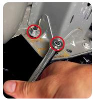
STEP 4: With the four 15mm nuts removed, move on to assembling the brackets that will hold the enclosure to the vehicle. Begin by attaching two of the rubber isolators to bracket "2" using two 10mm nuts.
