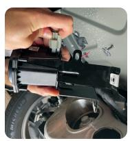
STEP 3: Next, remove the inside, factory bumper nuts. There will be two 15mm nuts on each side of the factory bumper in the cavity that was exposed earlier. Remove all four nuts to prepare to mount the enclosure brackets.
