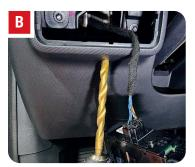
Feed the 4 pin connector end through the 1/2 inch hole and pull through (A). Then, using a wire snake or similar, route the 4 pin connector end down to the driver side kick panel area (B).
