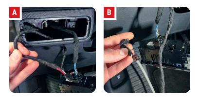
**STEP 3:** Next, using a small screwdriver, position the Controller in place and mount it to the dash using the two provided screws.
