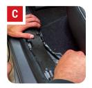
STEP 2: Next, move to the driver side front of the vehicle to remove a few panels to continue the Speaker Wiring Harness routing. Using a panel removal tool or similar, remove the panel on the side of the dash (A). Then, remove the small trim panel below the A pillar (B). Next, you will remove the driver side door sill panel.
