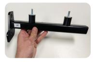
STEP 5: Next, assemble brackets "4" and "5" together using three 10mm nuts and the shorter bolts. Then, attach bracket "2" with the rubber isolators to the bracket "4" and "5" assembly using two of the provided 10mm nuts.
