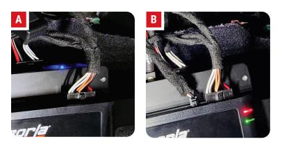
**STEP 5:** Finally, connect the 2 pin white connector from the Data Wiring Harness to the previously ran Speaker Wiring Harness in the driver side kick panel area.
