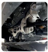
Next, remove the factory alert speaker. Remove the two 10mm bolts holding the factory STEP 2: alert speaker to the under body of the vehicle. Unplug the speaker and set aside.
