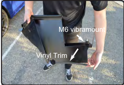
10. Install the provided Vinyl trim to the bottom of the heatshield. Install the M6 vibramount to the Thredded insert on heatshield.
