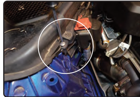
12. Loosen the T30 torx screw located near Postive battery terminal. Save bolt for later install.
