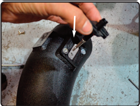
19. Re-install the temp sensor into the new injen intake tube and secure using the provided M4 button head screws.
