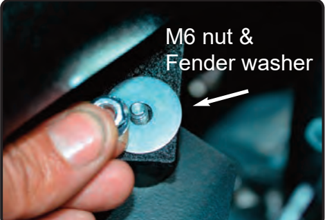
22. Secure the bracket on intake tube using provided M6 nut and fender washer. Tighten using 10mm socket or wrench.
