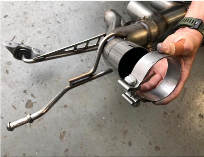
**27. (MUFFLER DELETE ONLY)** Locate the CORSA NPP valved muffler delete assembly, and the two supplied 3" clamps from the hardware kit. Position both clamps on the pipe inlets, so the clamp bolts are on the outside of the expansion and facing downwards as shown.
