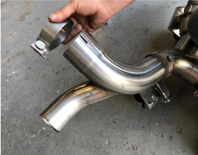
**11. (FULL MUFFLER ONLY)** Locate the two supplied 3" clamps. Position both clamps on the center crossover pipe inlets, so the clamp bolts are on the outside of the expansion and facing downwards as shown.
