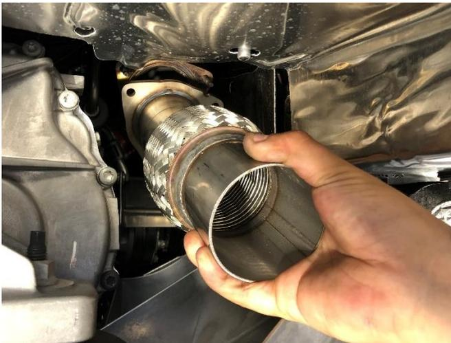
**1.** Locate the CORSA passenger side head pipe assembly, and the three M8 nuts set aside in **REMOVAL STEP 23**. Insert the passenger side CORSA head pipe assembly onto the studs from the catalyst as shown, then hand tighten the M8 nuts to hold the head pipe in place. Note the position of the head pipe assembly within the chassis when it is correctly positioned.
