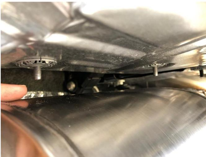
**25. (FULL MUFFLER ONLY)** Adjust the muffler position as needed until there is approximately a fingertip clearance between the heat shielding mounting studs and the top of the mufflers on both the driver and passenger side.
