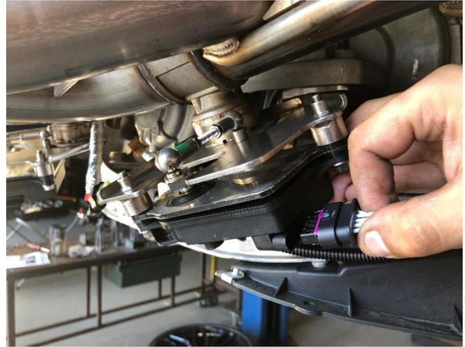
**35.** Connect the opposite end of the wiring extensions to the NPP valve actuators on both sides of the vehicle. Push in the grey locking tabs on the wiring connectors to secure the connections.
