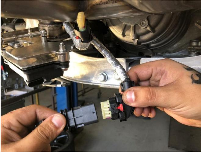
**34. (ALL VERSIONS)** Locate both supplied NPP valve wiring extensions. Connect both wiring extensions to the chassis side of the NPP valve wiring connectors. Push in the grey locking tabs on the wiring connectors to secure the connections.
