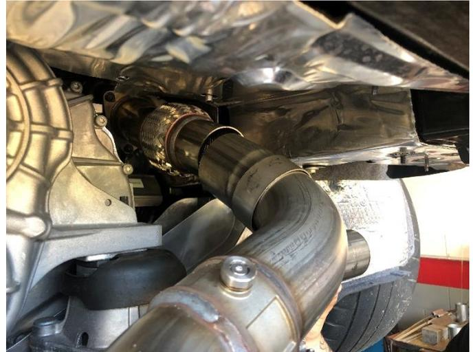
**12. (FULL MUFFLER ONLY)** Insert both inlet connections of the CORSA center crossover assembly on to the outlets of both head pipe assemblies, with approximately 1.75" of overlap at the pipe connection on both sides.
