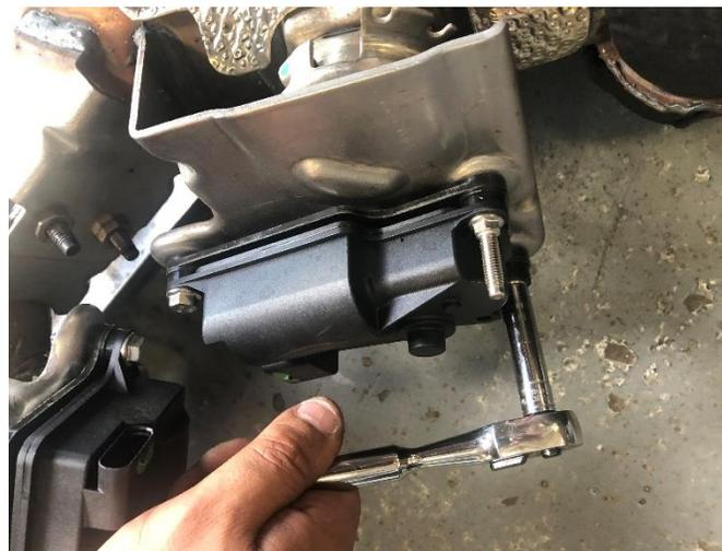
**31.** Repeat **REMOVAL STEP 30** for the driver side factory NPP valve actuator using a 10mm socket and a 1/4" ratchet for the one bolt and an 8mm socket and a 1/4" ratchet for the two studs. Label and set aside the NPP valve actuator in a protected location. Both NPP valve actuators will be reused during the installation of the CORSA exhaust system.
