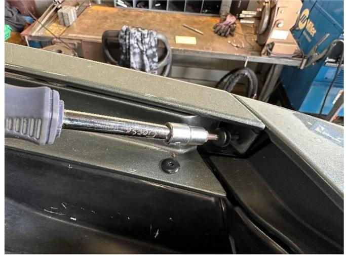
**17.** Remove the last two T15 TORX screws that are facing rearward and tucked into the corner of the fender on each side. This will allow the bumper cover to move independently from the vehicle. Set aside the fasteners in a protected location.
