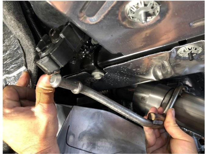
**28. (MUFFLER DELETE ONLY)** Insert both the driver and passenger side muffler delete front hangers into the front exhaust grommets as shown.
