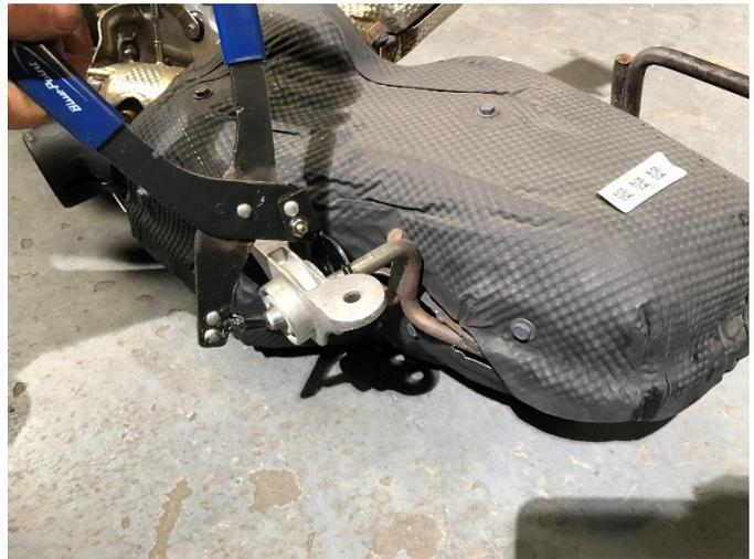
**27.** Remove both rear exhaust grommets from the exhaust hangers using grommet pullers or similar device. Note the orientation of the grommets for the installation of the CORSA exhaust system. Set aside the grommets in a protected location.
