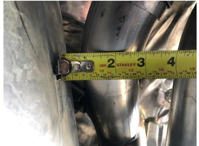
**14. (FULL MUFFLER ONLY)** Adjust the rotation and overlap of the center crossover assembly onto both head pipes until the outlets are even vertically, and each of the center crossover pipe to muffler outlet connections have approximately 3/4" clearance from the front side of the pipe to the chassis as shown.
