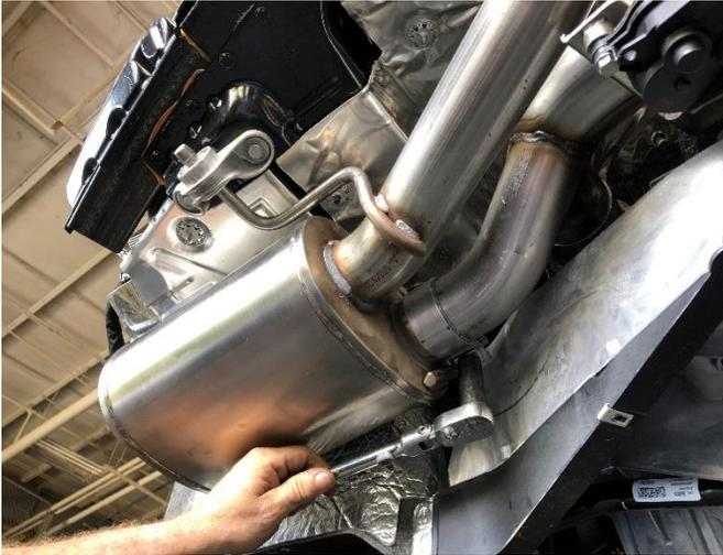
**23. (FULL MUFFLER ONLY)** Repeat **INSTALL STEPS 16-22** for the driver side of the vehicle (CORSA driver muffler shown), then remove the supporting jack stand from under the exhaust.
