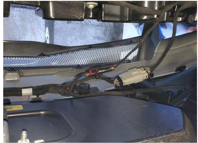
**19.** (Continued) followed by the two passenger side connectors to free the rear bumper cover from the vehicle. **CAREFULLY** set aside the factory rear bumper cover in a protected location.
