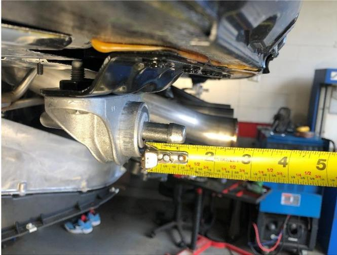
**31. (MUFFLER DELETE ONLY)** At this time, adjust the muffler delete and head pipe positions until there is approximately  $\frac{1}{2}$ " -  $\frac{3}{4}$ " between the outer face of the rear grommets and the forward edge of the head on the rear hangers on both driver and passenger sides of the vehicle as shown. It is critical for proper fitment to get the system adjusted as square as possible on the vehicle.
