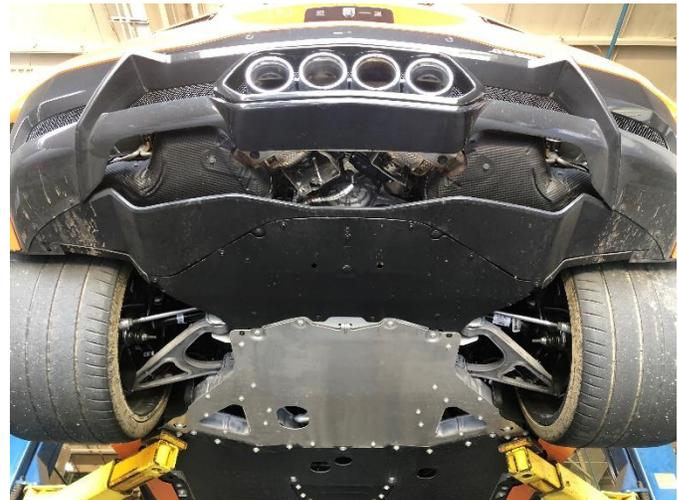
4. The rear bumper cover, two rear under trays, two inner fender liners, and the rear wheels will all need to be removed first in order to allow removal of the factory exhaust.
