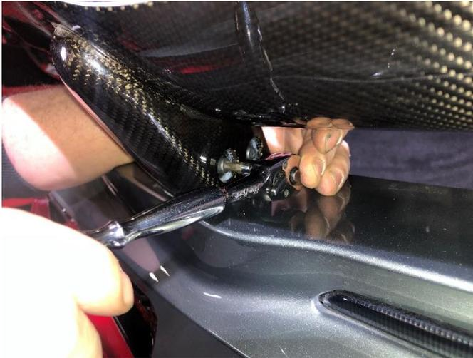
**13. (FOR Z07 PACKAGE ONLY)** Remove the four screws (2 per side) that secure the Carbon Fiber rear wing to the wing mounting blocks using a IPR30 TORX plus security bit and a ¼" ratchet...
