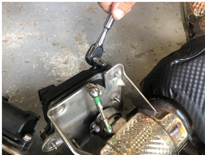
**30.** Remove the three bolts that secure the passenger side factory NPP valve actuator using a 10mm socket and a 1/4" ratchet. Label the passenger side actuator accordingly to ensure that it is properly identified for the installation process, then set aside the NPP valve actuator in a protected location.
