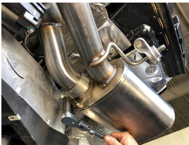
**22. (FULL MUFFLER ONLY)** Tighten the exhaust clamp at the passenger side muffler inlet connection using a 15mm socket and 3/8" ratchet to secure the passenger muffler assembly.
