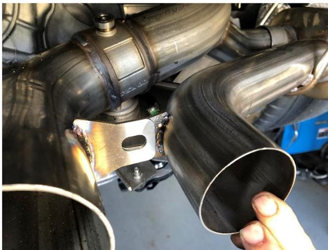
**19. (FULL MUFFLER ONLY)** Locate the supplied M10x20mm long flange bolt and M10 flange nut. Make sure the tie bracket from the passenger muffler assembly is positioned in front of the corresponding tie bracket on the passenger side of the center crossover assembly as shown.
