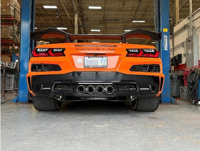
**37.** At this time, adjust the exhaust system position until all exhaust pipe outlets are centered within the collectors on the factory center exit tips, which are mounted to the rear valence.
