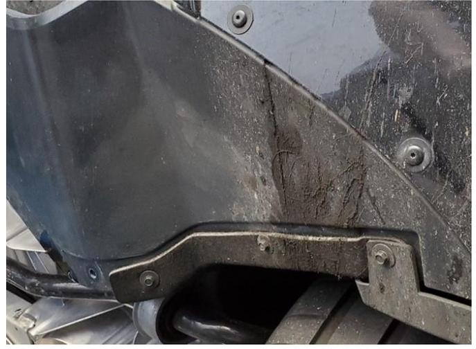
**6.** The rearward under tray is secured by two push clips (1 per side), four T15 TORX screws (2 per side), and six 7mm bolts (3 per side). Remove the push clips first using a removal tool or flathead screwdriver, followed by the T15 TORX screws, and then the bolts using a 7mm socket and ¼" ratchet. This will free the rearward under tray from the vehicle. Set aside the rearward under tray and fasteners in a protected location.
