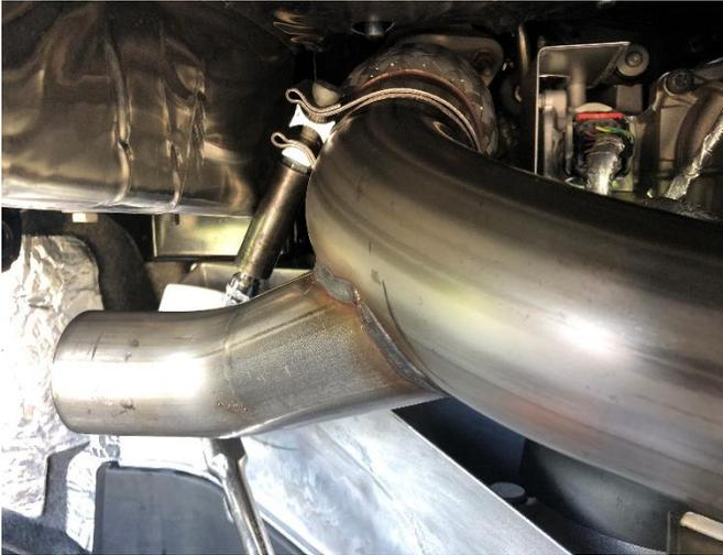
**15. (FULL MUFFLER ONLY)** Tighten both exhaust clamps at the driver and passenger side center crossover inlet connections using a 15mm socket and 3/8" ratchet to secure the center crossover assembly.
