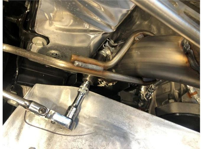
**32. (MUFFLER DELETE ONLY)** Tighten both exhaust clamps at the driver and passenger side muffler delete inlet connections using a 15mm socket and  $\frac{3}{8}$ " ratchet to secure the muffler delete assembly.
