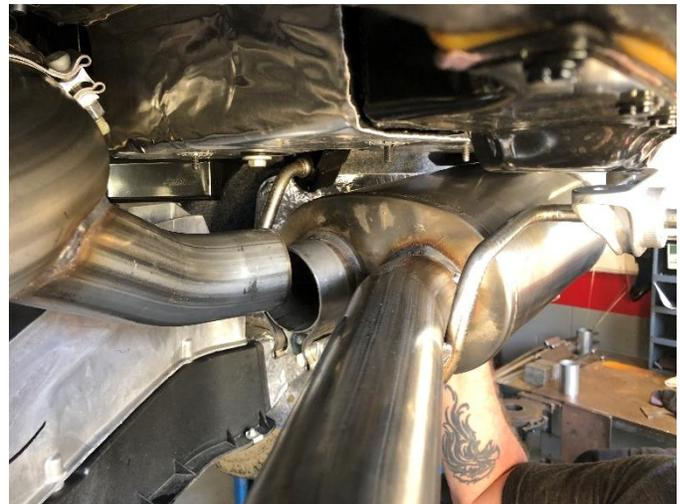
**18. (FULL MUFFLER ONLY)** Insert the inlet of the passenger muffler assembly on to the passenger side outlet of the center crossover assembly with approximately 1.375" of overlap.
