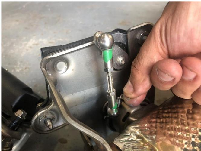
**28.** Remove the two locking pins from both NPP valve actuator linkages on the factory valve side (not valve actuator side) of the linkage as shown....
