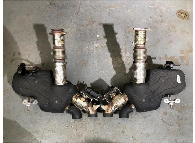
**25.** CAREFULLY slide the factory exhaust down and rearward to free it from the vehicle.
