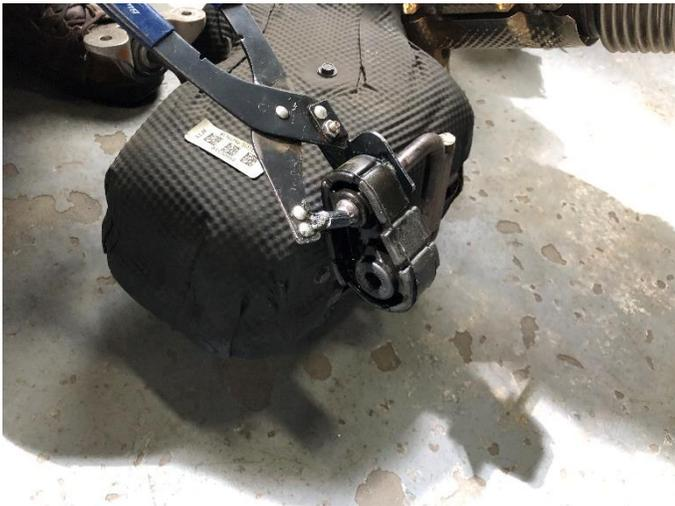
**26.** With the factory exhaust on the ground, remove the front grommets from the exhaust hangers using a grommet puller or similar device. Once again, the use of a soap and water solution will aid in the removal of the hangers from the factory grommets. Note the orientation of the grommets for the installation of the CORSA exhaust system. Set aside the grommets in a protected location.
