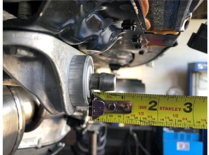
**24. (FULL MUFFLER ONLY)** At this time, adjust the muffler, center crossover, and head pipe positions until there is approximately  $\frac{1}{4}$ " between the outer face of the rear grommets and the forward edge of the head on the rear hangers on both driver and passenger sides of the vehicle as shown. It is critical for proper fitment to get the system adjusted as square as possible on the vehicle.
