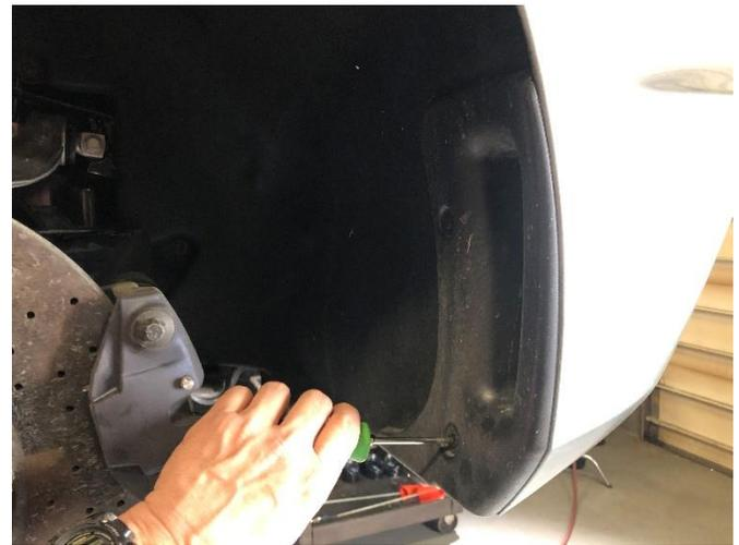
**8.** The two splash guard panels are secured by four T15 TORX screws (2 per side). Remove the screws to free the splash guard panels from the outside rearmost corners of the inner fender liners on both sides of the vehicle. Set aside the panels and fasteners in a protected location.
