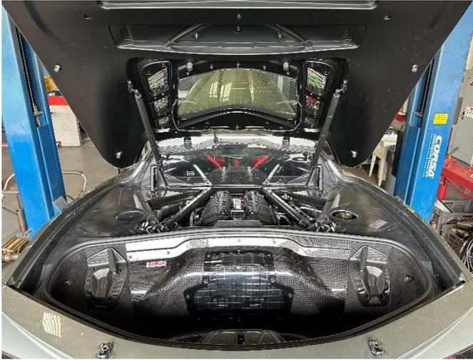
**16. (ALL VERSIONS)** Remove the sixteen T15 TORX screws that secure the top of the factory rear bumper cover to the chassis. Start with the fourteen screws that run along the top edge of the bumper.
