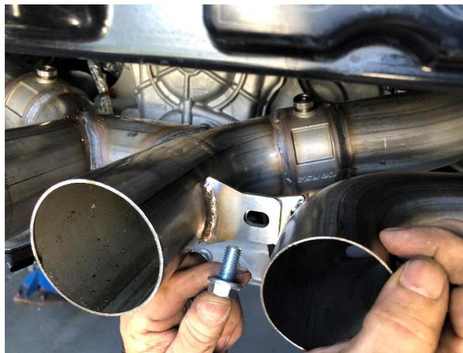
**20. (FULL MUFFLER ONLY)** Insert the M10 flange bolt through both slots in the tie brackets from the rearward side, and secure with the M10 flange nut. Snugly tighten with two 15mm wrenches, leaving it loose enough for later adjustment.
