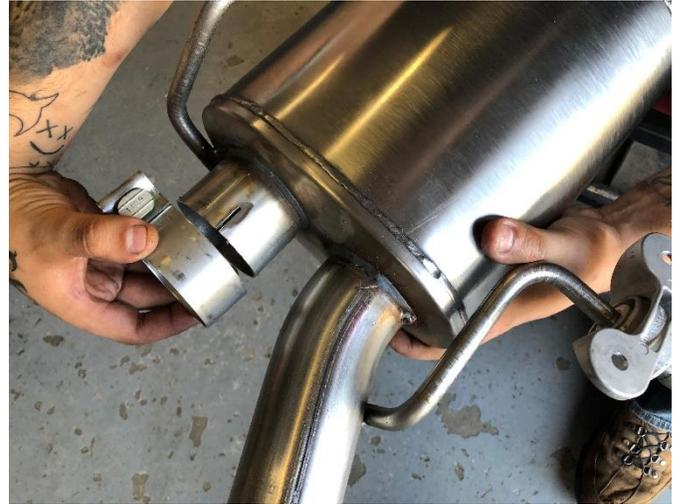
**16. (FULL MUFFLER ONLY)** Locate the CORSA passenger muffler assembly, and a supplied 2.5" clamp. Position the clamp on the passenger muffler inlet so the clamp bolt is in front of the expansion and the clamp nut is facing downwards.
