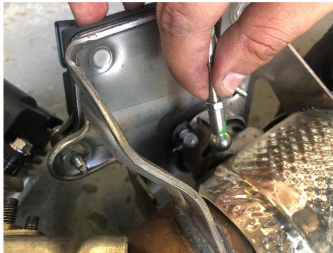
**29.** (Continued) then remove both NPP valve actuator linkages from the factory NPP valves as shown. Set aside the locking pins in a protected location.
