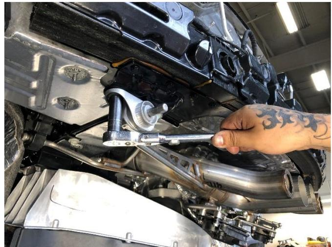
**30. (MUFFLER DELETE ONLY)** Locate the four factory rear grommet bolts set aside in **Removal Step 21**. Insert both bolts through the driver and passenger rear exhaust grommets and secure the grommets to the chassis using a 13mm socket and 3/8" ratchet. Torque to 17 FT-LBS.
