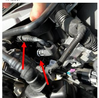
3. Locate the PCV line on the driver's side of the engine just behind the throttle body. Remove by pressing on the grey tabs on the PCV line fittings and pulling out.
