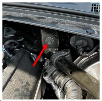
Locate the bolt found above the driver's side strut brace and remove using a 10mm socket.
