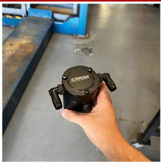
Thread in barbed fittings to the catch can ports by hand or by using an 11/16" wrench.
