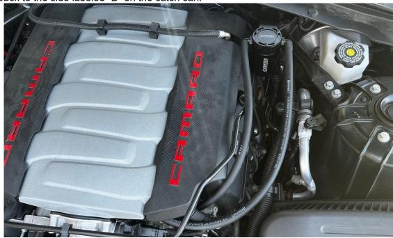
**6.** Make sure all fittings are secured in place and hose is pushed all the way over the barbed ends of the fittings. Reinstall engine cover and reclip fluid line above the engine cover.
