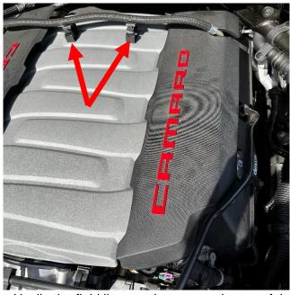
Unclip the fluid line running across the top of the engine cover. Remove the 2 side engine covers by pulling up and releasing them from the press fit tabs.
