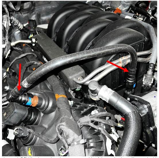
1. Remove the stock PCV line located on the passenger side of the engine by pulling on the blue tabs.
