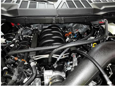
3. Install quick disconnect fittings to one end of each hose (Hose A gets the elbow fitting and hose B gets the straight fitting). Attach hose A to the A end of the catch can and route the hose to connect it to the BROWN fitting on the engine. Connect Hose B to the "B" side of the catch can and route the line to connect it to the BLACK fitting on the engine. Make sure fittings are fully secured and the hose is pushed all the way over the ends of the fittings.
