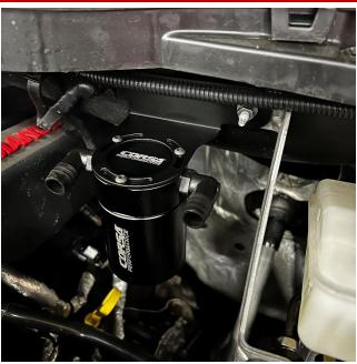
Locate the bolt and nut on the driver's side firewall that holds the coolant reservoir. Remove the nut using a 10mm socket and install catch can and secure it by reinstalling the nut.
