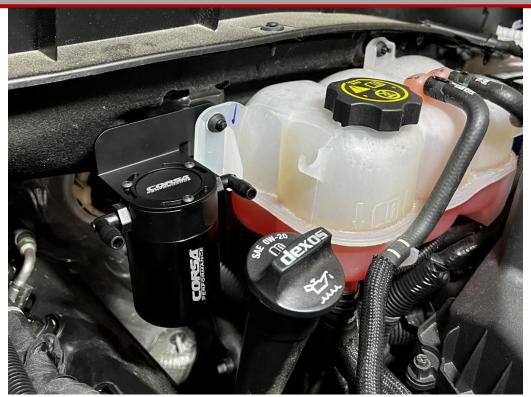
**5.** Make sure the nut is tight enough so the catch can is secure in place. Push the coolant reservoir back over the bolts on the firewall and tighten the bolt that was loosened.
