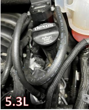
**6.** Connect the shorter Hose A to the "A" side of the catch can and route it to the fitting coming out of the crankcase. Connect the longer Hose B to the "B" side of the catch can and route the line to the fitting going to the intake manifold. Make sure all quick connect fittings are secured in place and hose is pushed all the way over the barbed ends of the fittings.
