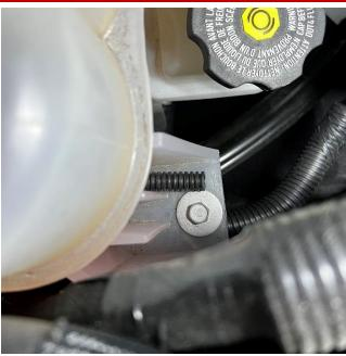
Use a 10mm socket to loosen the bolt holding the coolant reservoir on the driver's side of the engine bay up near the firewall.
