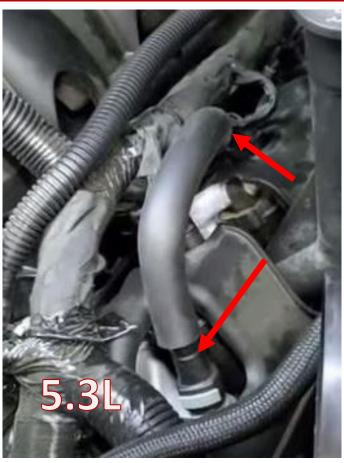
Locate the stock PCV line and remove the quick disconnect fittings by pressing on the grey tabs and pulling.
