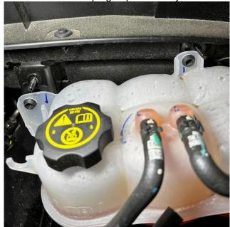
**3.** Once the bolt is loosened, pull the coolant reservoir from the two bolts extending out from the firewall.
