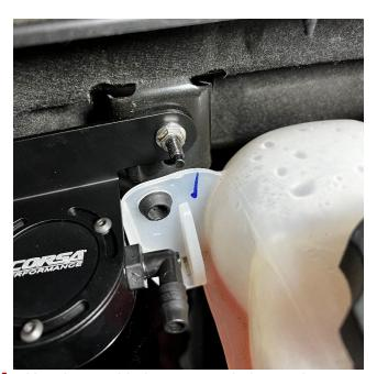
4. Use the provided nut to attach the catch can bracket to the coolant reservoir bolt.
