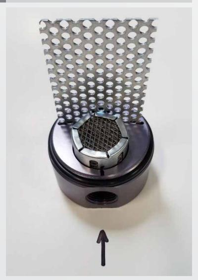
As seen in picture the arrow is pointing to the draw side make this side of the oil separator goes to the intake manifold. This helps filter the oil vapors through the screen and filter assembly.
