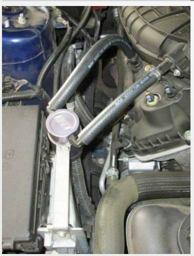
Before assembling kit notice that the shorter hose is going to the right which is your manifold draw. Remove factory computer mounting bolt now install kit and tighten down bracket bolt and supplied hose clamps at engine connections. (NOTE) some models the machined BBK logo are up-side down we have supplied a center BBK logo decal so you can install it for your desired look.
