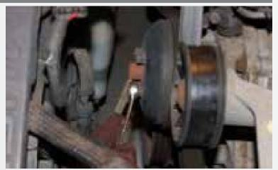
Loosen the bolts on the water pump and crank pulleys.
