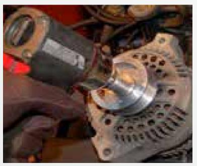
Remove the alternator mounting bolts, lift the alternator out of its cradle to access the pulley. Using an impact, remove the stock pulley and install the BBK Pulley. Re-use the stock nut and/or washer.
