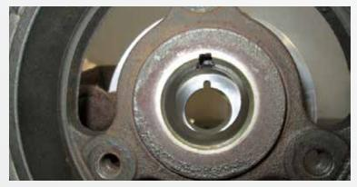
Install the hub of the factory harmonic balancer pulley into the counter bore of the BBK Pulley. Align the threaded hole in each pulley together. Install and hand tighten the (3)  $\frac{1}{4} \times 1-\frac{1}{4}$ " bolts. The factory pulley does not completely sit into the under-drive at this point. Carefully tighten the (3) bolts equally in small increments to draw the (2) pulleys together. Remove the (3)  $\frac{1}{4}$ " bolts.
