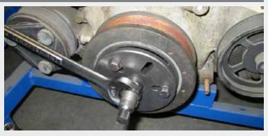
Remove the center bolt and washer from the factory pulley/dampener. Remove the alternator pulley and water pump pulley. Use a 3 prong harmonic dampener puller to remove the factory pulley/balancer. cont. next column
