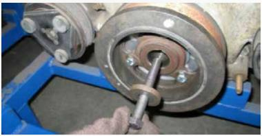
Attach the pulley assembly to the crankshaft using the new bolt provided and the original crank bolt washer. Use locktite or equivalent on the bolt and torque to 60 ft/lbs. Install the new water pump pulley using the original hardware. Also use locktite.
