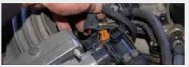
Unplug the TPS and IAC valve electrical connections.
