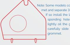
Note: Some models come with a large rubber grommet and separate 3-1/2" diameter tube assembly. If so install the large grommet into the corresponding hole in the fender-well bracket, lightly oil the grommet inside diameter and carefully slide the 3-1/2" tube through the grommet.
