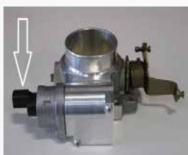
Using the new gasket and hardware supplied in the kit assemble the IAC valve and adapter to the BBK Throttle Body.
