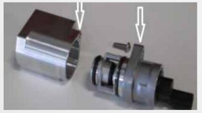
To install the IAC valve into the supplied adapter. Line up the bolt holes and press the IAC valve into the adapter supplied in the kit. Using the supplied bolt tighten it down to secure the two pieces together.
