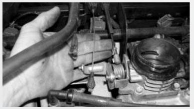
Unclip the cable attachments from the throttle linkage.
