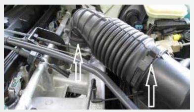
Loosen the (2) clamps that hold the air inlet tube to the throttle body and the air box.
