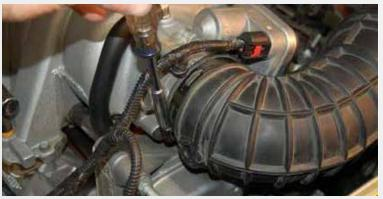
Unplug the air temperature sensor on the stock inlet tube. Remove the sensor for re-use in the BBK inlet tube. Loosen the clamp at the throttle body.
