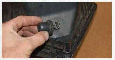
On the bottom rear of the stock air box, remove the rubber grommet for reuse with the BBK filter shield.
