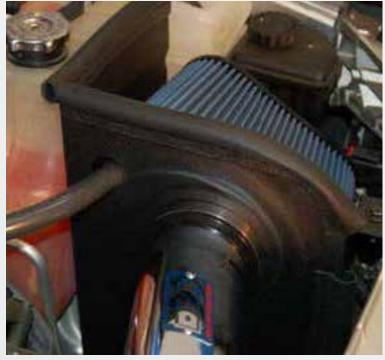
Place the supplied filter into the shield area and push the neck of the filter base, where the clamp mounts, through the opening in the filter shield. Install the BBK Inlet Tube into the filter and into the blue hose connector. Position for the best fitment and be sure the opening in the base of the filter lines up with the smaller hole in the filter shield. Then tighten the clamps.
