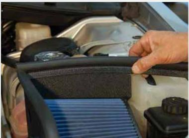
From the supplied hardware kit, find the aluminum pin and 1/4" Phillips screw and install on the BBK filter shield. Install the stock rubber grommet onto the pin. Install the supplied sponge rubber seal to the top of the filter shield.
