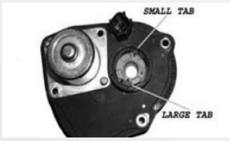
Using needled nose pliers, rotate the plastic spring cap COUNTER-CLOCK-WISE (approximately 180 degrees) until the 2 tabs line up with their matching landings in the motor housing, then gently pull up on the cap until it pops up into a latched position.
