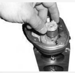
Place the plastic capped spring over the end of the throttle shaft of the BBK Throttle Body and line the pig tail hook on the spring up with the catch slot in the gear.
