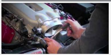
Remove the 4 bolts that hold the throttle body to the intake manifold.
