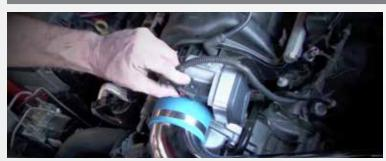
Re-connect the air temperature sensor and the throttle body control motor plug. Re-connect the negative battery terminal and refer to page 2 of the instruction sheet for throttle relearn procedure.
