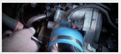
Loosen the clamps on the air intake tube and air box, and then remove the tube.
