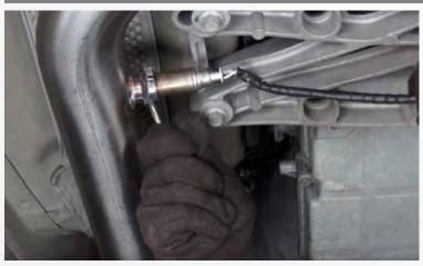
Remove the oxygen sensors from the stock pipes and install onto the BBK Mid-Pipes.
