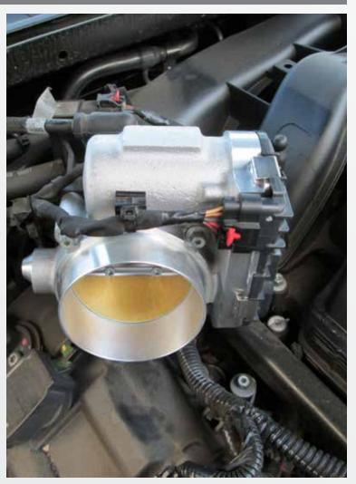
Now bolt on BBK throttle body re-using stock hardware making sure to not over tighten stock bolts.
