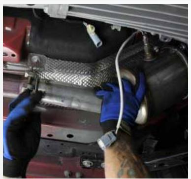
Install the stock catted down pipe back onto the exhaust line up the catted down pipe to the new flange and snug down the coupler that connects the mid pipe to the resonator, then just snug down the ball flare clamp enough so that you can still rotate the catted down pipe and align it with the hole in the flange.
