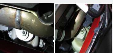
Remove the air filter box. Remove the first and second nuts on the top row of studs on the stock header of the driver side. On the passenger side, remove the first top nut that is behind the AC hose. Loosen the motor mount nut that faces up towards the header on each side, however do not remove completely at this time
