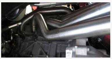
Install the supplied gasket and the BBK Header on the remaining studs and install the nuts and bolts. You may have to raise or lower the motor a bit to get the BBK header in place tighten all the nuts and bolts that you can reach from underneath the vehicle.
