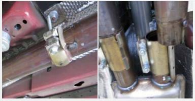
Loosen the ball flare clamp on the driver side pipe near the transmission cross member then loosen the exhaust coupler at the resonator and remove the driver side pipe from the vehicle.
