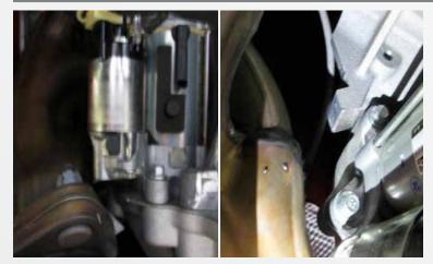
Remove the ( 3) 10mm bolts that hold the starter in place then remove the starter and hang it to the side.
