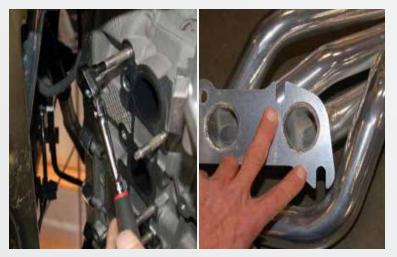
Using an 8mm Torx Bit socket remove all the exhaust manifold studs from the engine block except for the ones that correspond to the (2) notches in the BBK header flange that are closest to the firewall.
