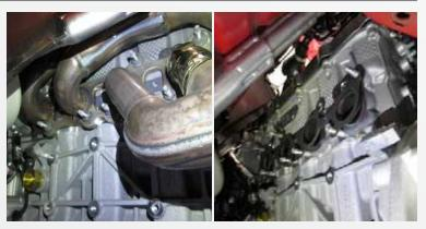
Remove the remaining exhaust manifold nuts then remove the exhaust manifold along with the gasket from the vehicle.
