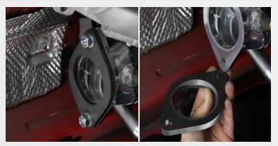
Using the supplied hardware install the supplied gasket and flange onto the BBK Tune length header. NOTE!!! Be sure to face the flange in the correct direction as pictured below.
