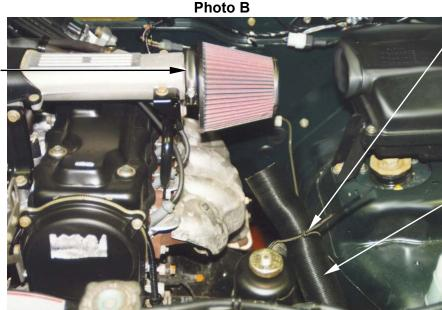
2. Lenghthen the flexi cold air hose to 32" / 81cm. Tie the flexi cold air hose to the PAS hose coming from the reservoir with the long plastic tie supplied.
