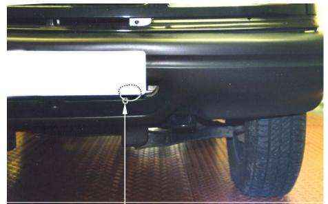
Feed the flexi cold air hose down towards the front L.H.S. lower grille, then pierce / drill a 3mm hole in the lower part of the bumper / grille and also in the end of the cold air hose. Attach the hose to the grille with the medium plastic tie.
