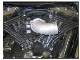
9. Install the K&N® intake tube onto the throttle body along with the provided gasket and secure with the provided mounting bolts.
