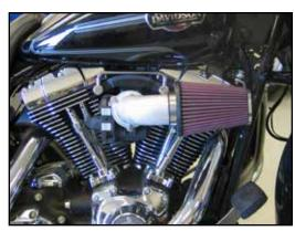
10. Install the provided K&N® air filter and secure with the provided hose clamp. A black hose clamp is being supplied with kit. This clamp is intended to clamp the filter to the intake tube.
