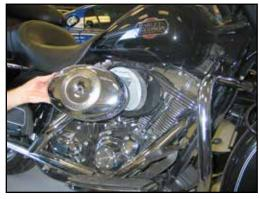
2. Remove the air filter cover bolt and air filter cover as shown.
