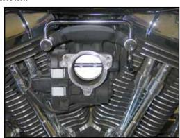
7. Install the supplied crankcase breather tube using the provided breather bolts and washers. NOTE: Place one washer on each side of the of the breather tube.
