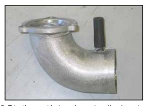
8. Trim the provided crankcase breather hose to a length of 1.5" and then install it onto the K&N® intake tube as shown.
