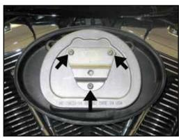
3. Loosen the three air filter retaining bolts shown.
