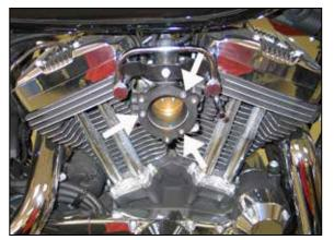
8. Install the K&N® intake tube adapter onto the throttle body using the provided hardware.
