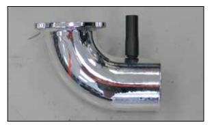
9. Cut the provided crankcase vent hose to a length of 1.75" and install onto the K&N® intake tube as shown.
