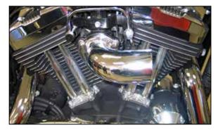
10. Install the K&N® intake tube onto the throttle body while attaching the vent hose to the vent tube and secure with the provided hardware. NOTE: Apply one drop of the provided thread locker to the K&N® intake tube mounting bolts, adjust the vent tube and intake tube/throttle body for best fit, and tighten the mounting bolts.
