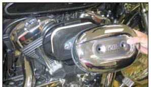
2. Remove the two air filter cover mounting bolts and then remove the cover from the vehicle as shown.
