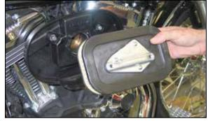
4. Remove the air filter as shown.
