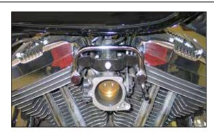
7. Install the K&N $^{\circ}$  crankcase breather tube onto the vehicle using the provided hardware. NOTE: Do not completely tighten the breather bolts at this time.
