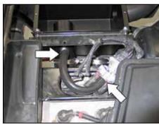
19. Install the provided idle by-pass hose onto the npt vent fitting and then onto the idle solenoid.
