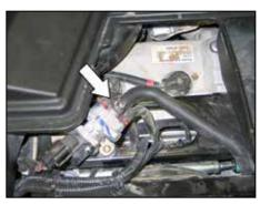
8. Loosen the hose clamp that secures the idle bypass hose to the idle bypass solenoid.
