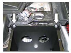
16. Secure the top of the air box to the mounting bracket with the provided hardware and then tighten the lower mounting nut and hose clamp securing the fresh air intake hose.
