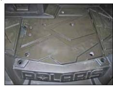
23. Reinstall the engine access panel.
