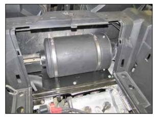
17. Install the filter canister assembly onto the mounting tray and connect the fresh air inlet hose. Adjust the canister and hose for best fit and then secure the canister and hose with the hose clamps. NOTE: Due to differences in the production factory foil heat shield, the heat shield may need to be reformed to allow the canister and
