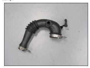
20. Remove the inlet temperature sensor from the factory intake tube.
