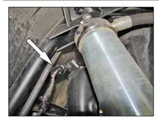
7. Release the clip securing the inlet temperature sensor electrical connection and then disconnect the sensor electrical connection.
