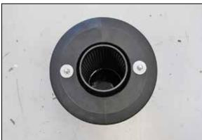
15. Install the filter assembly into the K&N® filter canister and secure with the provided hardware.
