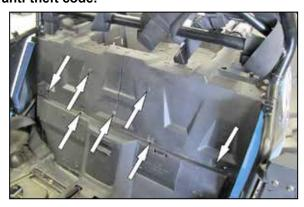
2. Release the locking leaver and Remove the (rear) seats from the vehicle and set aside. Remove the eight bolts shown that secure the rear panels.
