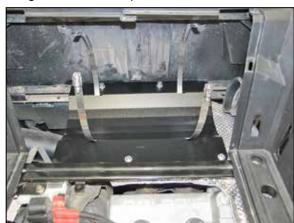
11. Install the filter base plate assembly as shown using the provided hardware.
