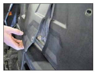
3. Pull back the inner lower corners of the back panels to gain access and remove the two air filter housing mounting bolts.
