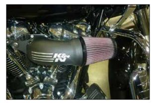
12. Install the K&N® air filter onto the intake tube and secure with the provided hose clamp.
