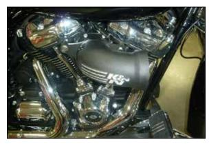
11. Install the K&N® intake tube with the gasket and provided hardware.
