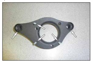
8. Install the remaining two o rings onto the front of the back plate as shown. Install the three provided studs with thread locker positioned into the back plate.
