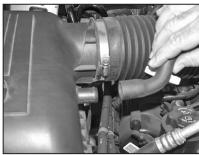
2a. On vehicles equipped, disconnect the crankcase vent from the airbox as shown.
