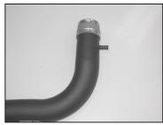
23. Install the provided silicone hose (08051) onto the K&N® intake tube with the provided hose clamp as shown
