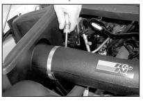
27. Using the provided hose clamp, secure the K&N® intake tube to the saddle bracket assembly as shown.
