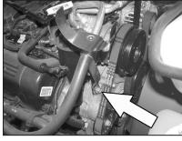
21A. On vehicles equipped with a bracket between the belt tensioner and the a/c compressor, install the provided spacer between the supplied bracket and factory bracket.
