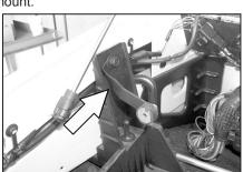
19. Install the twisted "L" bracket with the bolt that was removed in step 18. Do not tighten bolt completely.
