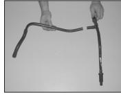
32. Cut the crankcase vent tube 1" from the "T" fitting as shown
