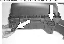
10. Remove the two rubber bushings from the factory airbox as shown.
