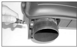
25. On models that come equipped with temp sensors, remove the air temp sensor from the resonator box as shown.
