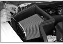
37. Align the heat shield for best clearance then tighten all the brackets.
