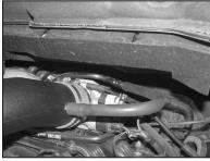
35. Connect the provided vent hose onto the "T" fitting, then connect the other end onto the K&N $^{\circ}$  intake tube.
