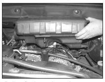
6. Pull up firmly to release the resonator from the engine.
