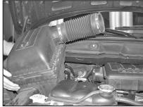
3. Lift firmly to release the airbox from the mounting studs, then remove completely.
