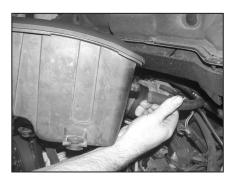
7. On 2007 and earlier model vehicles, disconnect the crankcase vent hose from resonator box as shown, then remove resonator box from vehicle.
