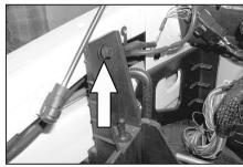
18. Remove the 8mm bolt that retains the airbox
