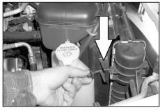
16. Remove the 13mm bolt from the upper fan shroud as shown.
