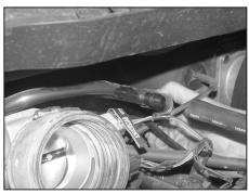
8. On 2007 and earlier model vehicles, remove crankcase vent hose from tee as shown.
