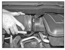
2. Loosen the hose clamp that connects the intake tube to the resonator box then remove the intake tube.
