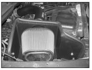
36. Install the K&N® air filter onto the K&N® intake tube as shown and secure with the hose clamp.
