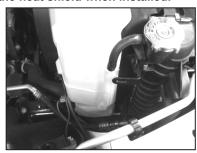
16B. Install the "L" bracket (26607) onto the fan shroud with the provided 8mm bolt and washers.
