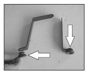
11. Install the two rubber bushings that were removed in the previous step into the provided brackets as shown.
