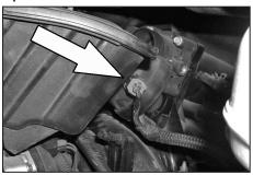
4a. On 2008 and later model year vehicles the inlet air temperature sensor is located on the driver's side of the vehicle next to the throttle body.
