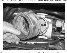
9. Loosen hose clamp that retains the rubber hose to the throttle body, then remove as shown.
