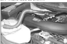
31. On models that the crankcase vent hose is connected to the "T" on the passengers side of the engine, remove the complete vent tube assembly from the rubber fittings in each valve cover as shown.
