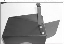
12. Install the large "Z" bracket onto the heat shield with the provided hardware. Do not tighten completely at this time.
