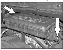
5. On 2007 and earlier model vehicles, remove the two 10mm bolts that retain the resonator box onto the engine
