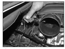
4. On vehicles equipped with a air temperature sensor in the resonator box, depress the locking tab and separate the electrical connection.
