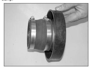
20. Install the silicone hose (#08051) onto the filter adapter and secure with the provided hose clamps as shown.
