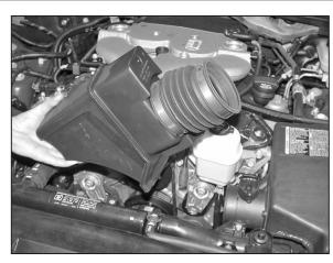
5. Loosen the two hose clamps on the intake plenum, then remove the intake plenum from the vehicle as shown.
