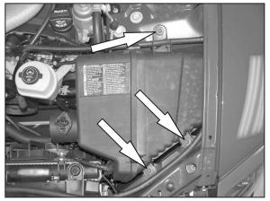
6. Remove the three bolts that secure the air box to the vehicle.
