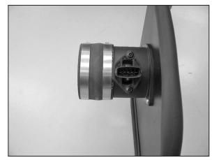
18. Install the silicone hose (#08690) onto the mass air assembly with the provided hose clamps as shown.
