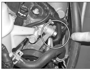
11. Remove the power steering pump mounting bolt shown with a 15mm wrench.
