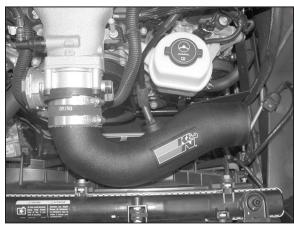
14. Install the new K&N® intake tube onto the throttle body and secure with the provided hose clamp. Secure the tube to the K&N® tube bracket with the hardware provided.
