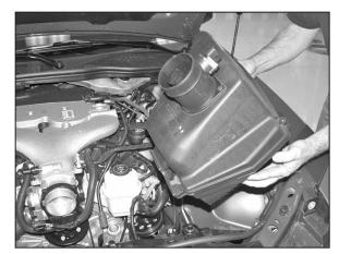
7. Remove the air box from the vehicle as shown. NOTE: K&N Engineering, Inc., recommends that customers do not discard factory air intake.
