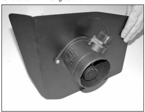
16. Install the mass air sensor onto the heatshield with the provided hardware as shown.
