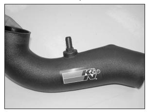
13. Install the provided NPT fitting onto the K&N® intake tube as shown.
