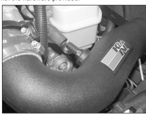
15. Install the crankcase vent hose onto the K&N<sup>®</sup> intake tube NPT fitting as shown.
