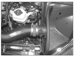
19. Install the heat shield assembly onto the K&N® intake tube and secure with the provided hose clamp.
