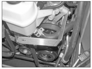
12. Install the K&N $^{\rm @}$  "L" bracket (#07188) as shown with the bolt removed in step #11.
