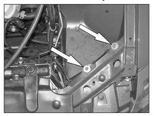
8. Secure the splash shield onto the vehicle with the provided hardware as shown.
