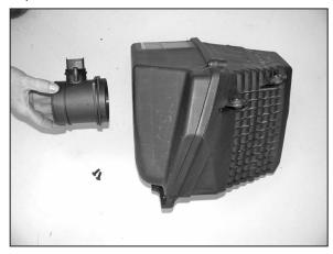
9. Remove the two screws that secure the mass air sensor to the air box, then remove the mass air sensor.
