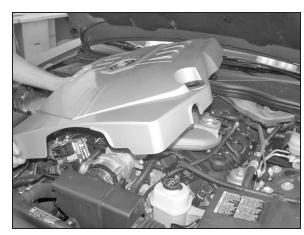
3. Remove oil cap, then pull up on engine cover to release from its retainers.
