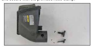
13. Remove the screws securing the Mass air sensor and Humidity sensor into the factory air box and then remove the sensors.
