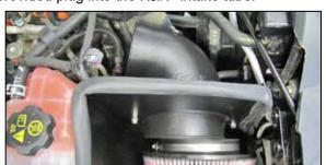
12. Install the K&N® intake tube into the heat shield and secure with the provided hardware and then install the K&N® air filter onto the K&N® intake tube and secure with the provided hose clamp.
