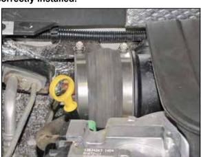
17. Install the provided hump hose (08633) onto the turbo inlet and secure with the provided hose
