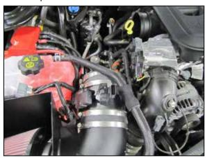
16. Install the Mass air assembly onto the K&N® intake tube as shown and secure with the provided hose clamps.
