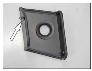
13. Install the heat shield mounting bracket (07805) onto the heat shield using the provided hardware and spacer.
