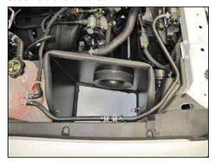
14. Install the heat shield into position and secure with two of the factory nuts removed in earlier steps.
