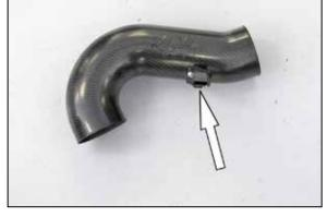
22. Install the mass air sensor into the K&N<sup>®</sup> intake tube and secure with the provided hardware.
