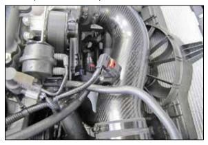
26. Reconnect the mass air sensor electrical connection.
