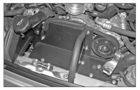
16e. Reinstall the heat shield assembly and secure with the provided inserted nuts and "L" bracket (070066). Secure the "L" bracket to body with the provided hardware.
