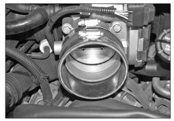
22. Install the silicone hose (08690) onto the throttle body and secure with the hose clamp provided.
