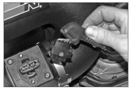
32. Pull the rubber wiring harness boot back from the mass air sensor electrical connection, rotate the connector 180° and reinstall the boot.
