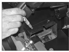
19. Mark the location of the holes in the heat shield on the fresh air supply duct as shown.
