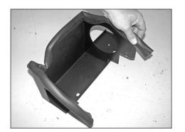
8. Install the edge trim onto the heat shield as shown.
