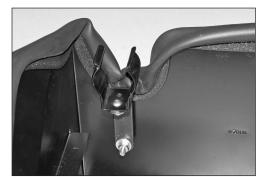
12. Using the spacer and hardware provided, install the oil filler tube retaining assembly onto the heat shield as shown.
