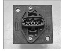
25.Using the hardware provided, install the mass air sensor onto the adapter plate as shown.
