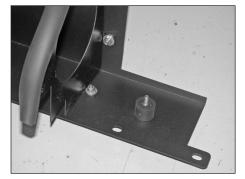
10. Install the rubber mounted stud onto the heat shield as shown using the hardware provided.
