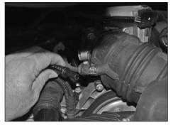
3. On "TIPTRONIC" equipped vehicles with a vent line connected to the stock intake tube next to the throttle body, loosen the hose clamp that secures the vent line and disconnect the vent line from the intake tube.
