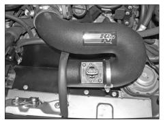
27. Install the K&N<sup>®</sup> intake tube onto the throttle body and saddle clamp, secure with the provided hose clamps.
