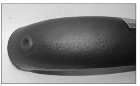
30. Remove the K&N<sup>®</sup> intake tube from the vehicle and drill a 3/4" hole at the marked location. Install the supplied grommet into the drilled hole. Be sure there are no shavings in the intake tube and then reinstall the K&N<sup>®</sup> intake tube into the vehicle and secure with the provided hose clamps. 35. Install the K&N<sup>®</sup> filter onto the intake tube and secure with the provided hose clamp. Snap the stock oil fill tube into the retaining clip.
