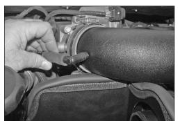
29. On "TIPTRONIC" equipped vehicles, install the 90° vent fitting assembled in step #28 onto the vent
