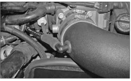
31. Install the  $90^{\circ}$  hose mender into the grommet installed in step #30 as shown.
