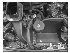
21. Using the hardware provided, bolt the fresh air supply duct to the heat shield as shown.
