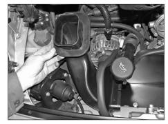
18. Install the fresh air supply duct into the heat
