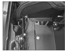
16f. Secure the heat shield to the "L" bracket (010040) installed in step 16e with the provided hardware.
