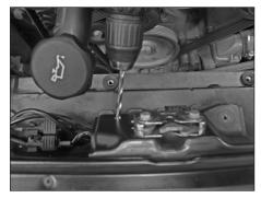
16c. Drill a 1/4"id hole into the hood latch support at the location marked in step 16b.
