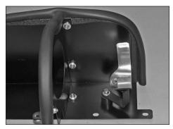
14. Install the saddle clamp assembly onto the rubber mounted stud on the heat shield with the hardware provided as shown.
