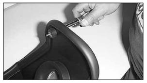
18. Attach the rubber mounted stud to the heat shield using the hardware provided. **Note: Do not tighten completely at this time.**
