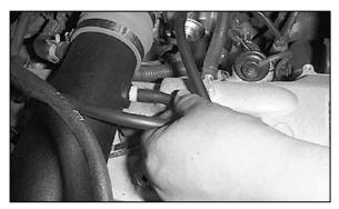
31. On models equipped with an A/C idle up magnetic valve vacuum line, attach the 1/4"id vent hose to the 1/8" barbed vent.
