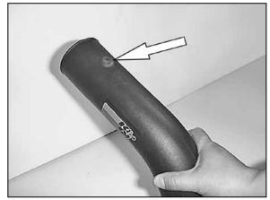
23. On models equipped with an external air temperature sensor, insert the grommet into the hole drilled in the previous step.
