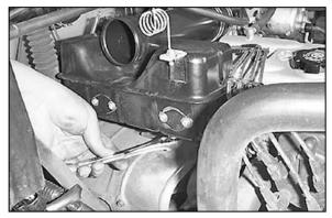
10. Loosen and remove the 2 nuts that retain the resonator assembly.
