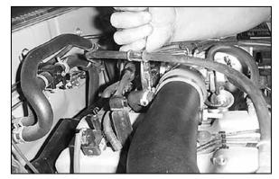
29. Attach the breather hose onto the vent on the intake tube.
