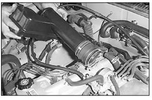
13. Loosen the hose clamp and remove the intake tube resonator assembly.
