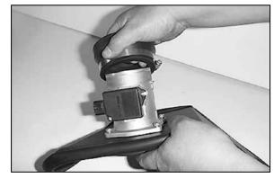
20. Install the tube adapter onto the flange of the mass air sensor and tighten hose clamp provided.
