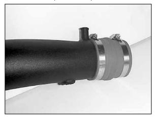
11. Disconnect the breather hose and A/C idle up magnetic valve vacuum line from the intake tube. Note: Not all vehicles are equipped with an A/C
