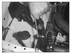
23. At this point, you can tighten the hardware located at the "L" and twist brackets as shown.
