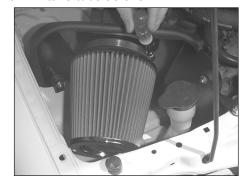
26. Install the K&N® air filter onto the mass air adapter and secure with the provided hose clamp as shown.
