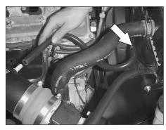
25. Install the provided silicone hose onto the EVAP canister vent and secure the other end onto the K&N® intake tube as shown
