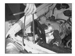
15. Install the heat shield assembly into the vehicle and secure it to the original air box mounting location as shown. Do not tighten completely.
