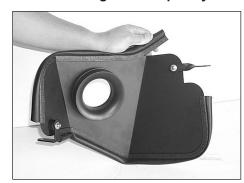
14. Install the twist bracket and the "L" bracket assembly onto the heat shield assembly with the provided hardware. Also install the trim seal onto the heat shield as shown.
