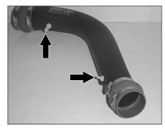
17. Install the two NPT fittings onto the  $K\&N^{\mbox{\scriptsize 8}}$  intake tube as shown.
