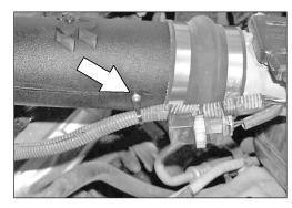
28. Secure the mass air sensor wiring harness to the intake tube with the tie wrap and screw provided.
