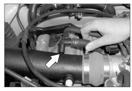
19. Vehicles equipped with an idle air vent line, install the 90 deg. fitting into vent line then mark the intake tube where the fitting lines up with tube. Vehicles that are not equipped with an idle air vent, continue on to step 23.
