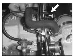
24. Install the provided silicone hose onto the fuel pressure regulator and connect the other end to the K&N® intake tube as shown.
