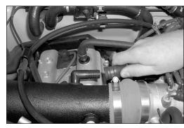
22. Vehicles equipped with the idle air vent line, reconnect vent line as shown.
