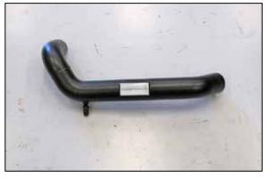
21. Install the provided vent fitting into the K&N® intake tube.
