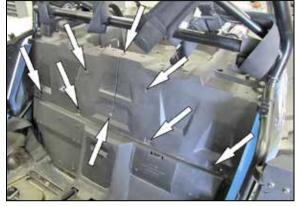
2. Release the locking leaver and Remove the (rear) seats from the vehicle and set aside. Remove the eight bolts shown that secure the rear
