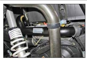
22. Feed the intake tube assembly behind the clutch intake hose and then install it into the intake plenum coupler and then into the filter coupler. Adjust the tube for best fit and then secure with the provided hose clamps.
