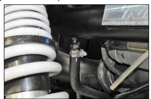
23. Install the crank case breather onto the fitting in the intake tube and secure with the factory clamp.
