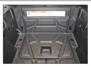
4. Release and lift off the engine cover.
