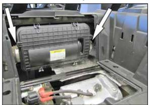
5. Loosen and remove the two hose clamps that secure the fresh air and clean air ducts to the air filter housing.
