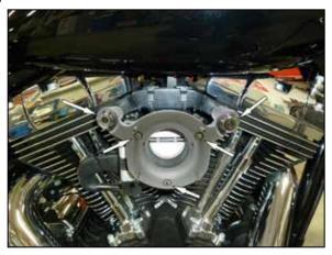
10. Using the two provided crankcase breather bolts; install the back plate onto the vehicle. Do not tighten bolts at this time. Install the provided gasket between the throttle body and back plate and then secure with provided hardware.
