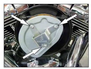
4. Loosen the three air filter retaining bolts as shown.
