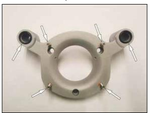
9. Install the remaining two o rings onto the front of the back plate as shown. Install the four provided studs with thread locker positioned into the back plate.
