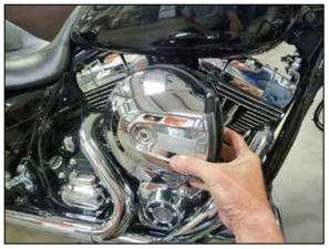
3. Remove air filter cover bolt and air filter cover as shown.
