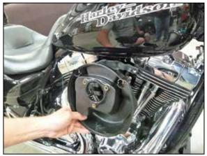
7. Remove the air filter base from the vehicle as shown.
