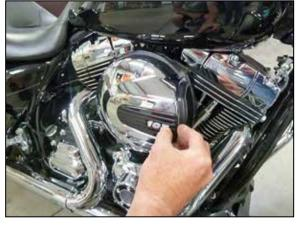
2. Some models have a number plate attached with Velcro. Firmly grip right side edge of number plate and pull off.
