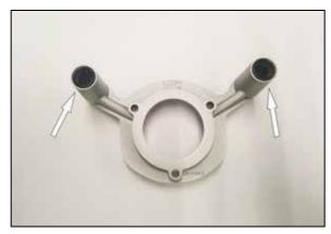
8. Install two of the o rings provided onto the back side of the K&N® back plate as shown.
