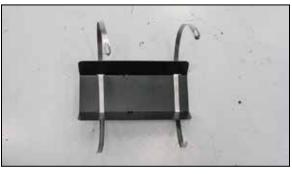
17. Install the two large hose clamps into the air filter housing mounting bracket as shown. **NOTE: the mounting bolts are off set to the left and the clamp adjusters are on the top in the photo.**
