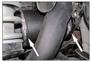
29. Adjust the air filter housing, turbo inlet hose and fresh air intake tube for best fit and then secure the hose clamps holding the air filter housing.
