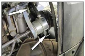
20. Install the K&N<sup>®</sup> intake hose assembly (084103) onto the turbo, rotate the hose so that the crank case vent hose aligns with the fitting installed into the K&N<sup>®</sup> hose. Install the crank case vent hose and secure with the factory hose clamp. Connect the vacuum hose to the fitting installed into the K&N<sup>®</sup> intake hose.
