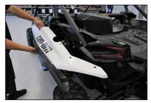
7. Remove the fender partially and then unhook the tail lamp harness from the fender and then completely remove the fender from the vehicle.
