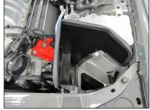
12. Install the provided coupling hose (KITHUMPHS12) onto the throttle body and secure with the provided hose clamp. Set the heat shield into position on the inner fender but do not secure at this time.
