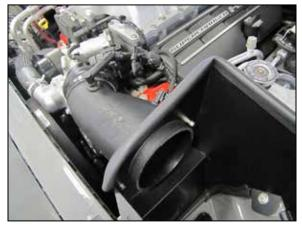
13. Install the K&N<sup>®</sup> intake tube into the coupling hose and heat shield and secure with the provided hardware to the heat shield.
