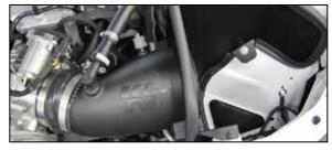
15b. Install the assembled crank case vent assembly onto the quick connect fitting installed into the K&N<sup>®</sup> intake tube and then connect the other end to the factory shut off valve and secure with the provided hose clamps.
